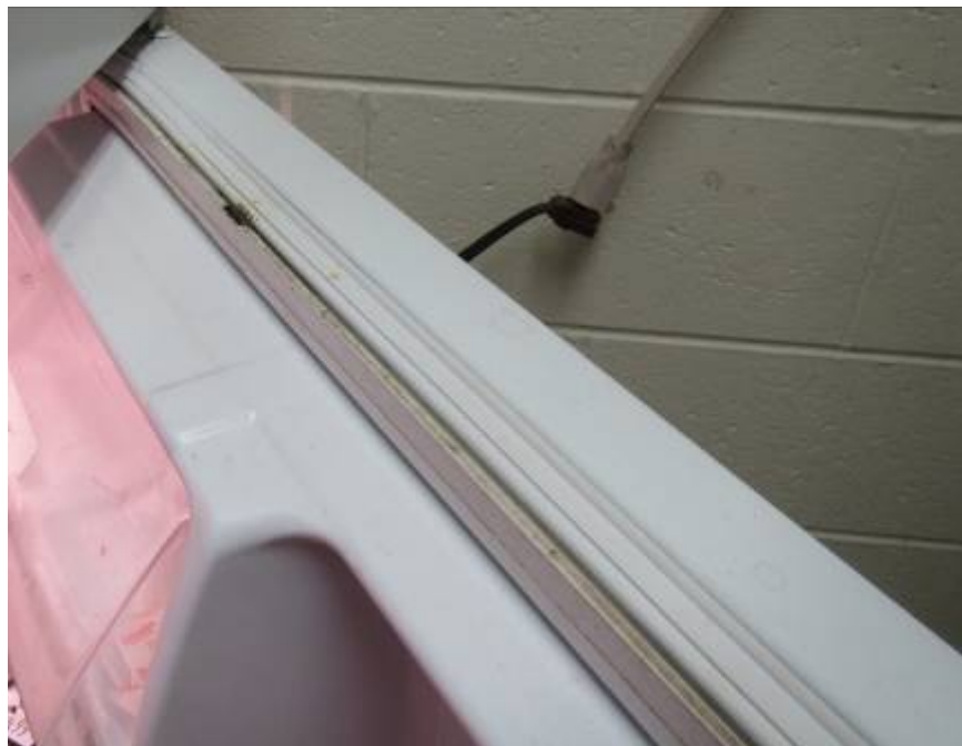
Refrigerator with dark staining/mold on gaskets
